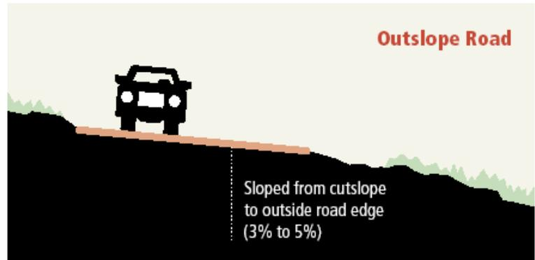
Outsloping, grade dips, open top culverts, and/or water bars can drain roads constructed on moderate slopes with light traffic loads. Though inexpensive to install, these methods may require frequent maintenance during periods of heavy use. This drainage method is not recommended on steep slopes or unstable soils for reasons of stability, safety and maintenance problems.
