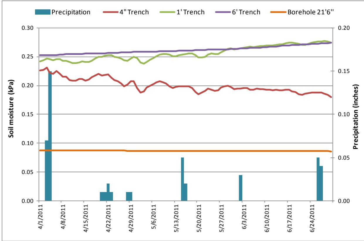
**Figure 2. Average daily soil moisture levels (kPa) at four depths and precipitation (inches) from the Tree site, April–June 2011.**
