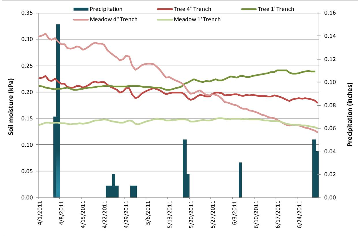
**Figure 5. Comparison of Tree and Meadow soil moisture levels at the 4-inch and 1-foot depths, along with precipitation, April–June 2011.**
